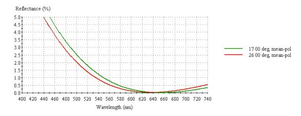
The reduction in reflection afforded by the AR coating over the uncoated surface of N-SF66 is a dramatic  $\sim$ 9.5% when optimising the layer thickness for each range. The reduction would not be so dramatic using a single coating as is intimated by the increasing slopes out of band in the curves above.
