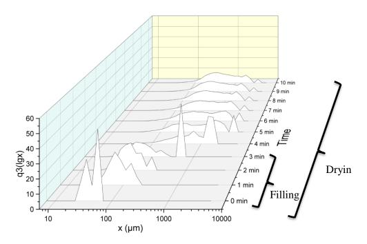
Figure 1. Volume density distribution q3 (lgx) with time, filling stage lasts for 3 minutes and total drying time is 10 minutes. 0 minute is defined as the time granules are detected by the probe.
