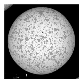
Figure 1. SEM picture of the patchy coated particle
