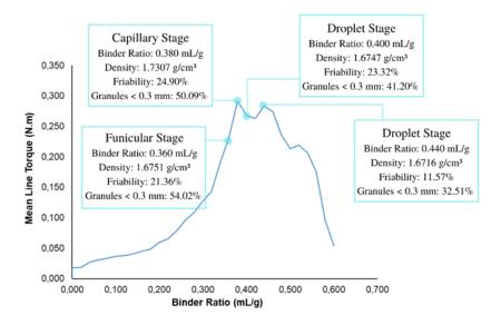
Figure 1. Rheological profile and granule characterization results for different binder ratios.
