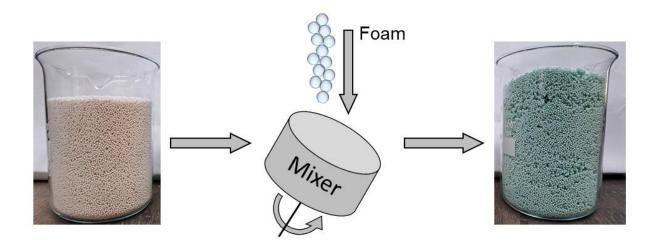
Figure 1. Foam coating of cellulose pellets
