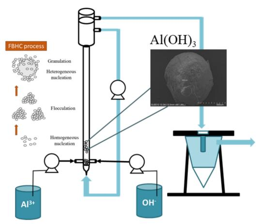
Figure 1. The concept of granulation by fluidized bed homogeneous technology (FBHC).
