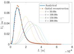
Figure 1. Time evolution of a volumetric particle size distribution subject to spatially homogeneous constant aggregation.
