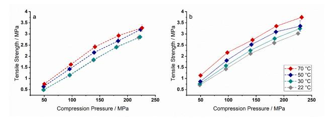
Figure 1. Change in tensile strength for different tableting temperatures. Binary blend containing lactose and (a) HPC SSL (b) HPC SSL-SFP ( $\bar{x} \pm sd$ , n=10).
