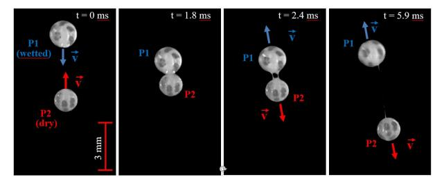
Figure 1. Wetted binary particle collision between two spherical  $ZrO_2$  particles with a diameter of 1.5 mm. The upper particle (P1) is wetted with a 116.3 µm thick layer of silicon oil with a kinematic viscosity of  $150 \cdot 10^{-6}$  m<sup>2</sup>/s at 20°C, while the lower particle (P2) is dry. The white particles are additionally marked with grey markers to track the rotation. They collide with a relative velocity in the normal direction of 1.57 m/s, which results in a complete rebound.
