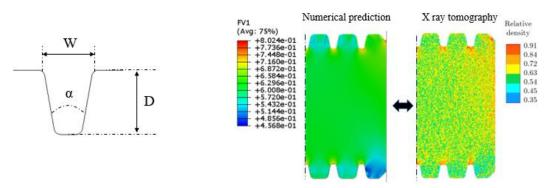
Figure 1. Groove shape (left), relative density distribution of grooved tablet (right)
