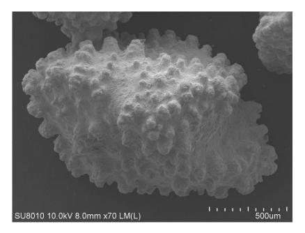
Figure 1. Recovery particle as zinc sulfide using fluidized bed homogeneous crystallization
