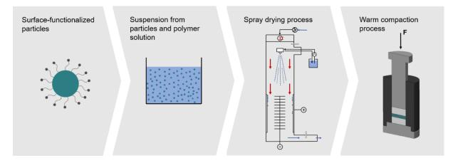
Figure 1. Process route for the production of composite pellets using functionalized particles by spray drying and warm compaction.
