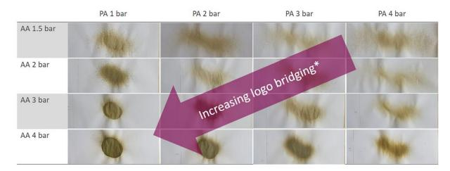
Figure 1. Images of Spray Characterisation with associated Atomization & Pattern air pressures
