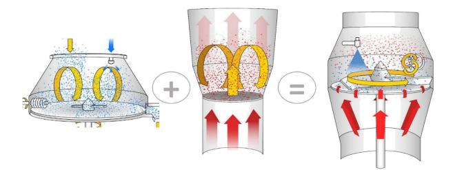
Figure 1. Schematic overview of fusion of traditional high shear granulation and fluidized bed drying into the TwinPro® process.
