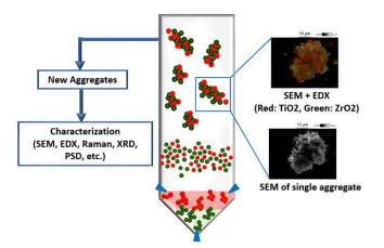
Figure 1. Experimental setup of the opposed-jet fluidized bed.
