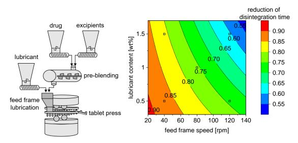
Figure 1. Schematic representation of the feed frame lubrication (left) and contour plot with disintegration time reduction for feed frame speed and lubricant content variations (right).
