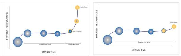
Figure 1. Drying curve of droplet temperature in conventional spray drying and electrostatic spray drying
