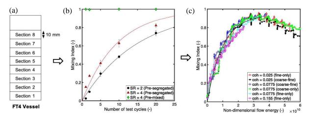
Figure 1. (a) the sectioned FT4 vessel used to assess mixing index (b) influence of particle size ratio on mixing rate (c) the developed relationship to predict mixing rate (black line) mapped against systems of varying cohesion
