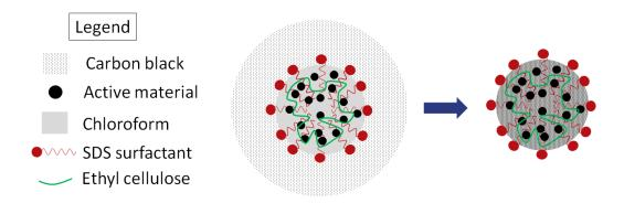
Figure 1. Mechanism of AM-CB co-agglomeration
