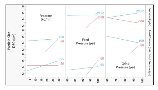
Figure 1. Particle Size D50 vs. Interaction Profiles generated via Fit Model
