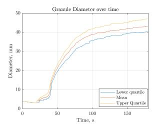
Figure 1. Granule growth behaviour within the DEM simulation, demonstrating induction growth and the distribution of sizes.
