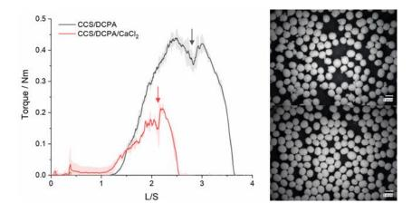
Figure 1. Mixer torque rheometry measurements of the two different mixtures (left) and the resulting pellets (top: CCS/DCPA (50:50), bottom: CCS/DCPA/CaCl<sub>2 (50:43:7)</sub>) at the optimal L/S (right)
