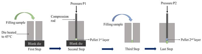
A schematic illustration of the pelleting process using a single-die pellet press.
