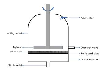
Figure 1. Cross-sectional representation of an AFD.
