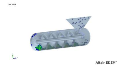
Figure 1. Particle Flow in Variable Density Extruder (VDE)
