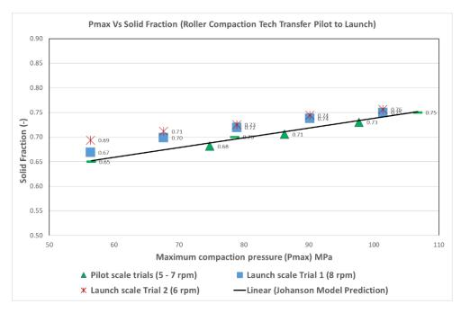
Scale up and tech transfer of roller compaction process - Pressure (Pmax) vs Solid Fraction.
