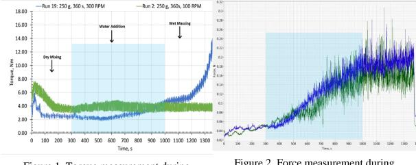
Figure 1. Torque measurement during granulation
