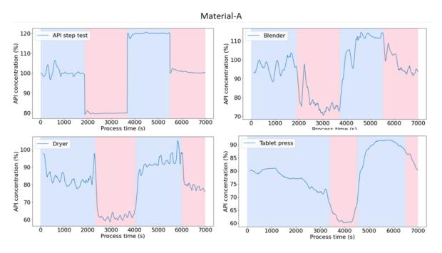
Figure 1. Graphical overview of the detection method for Material-A trials. Legend: background color changes symbolized the change point detection time.
