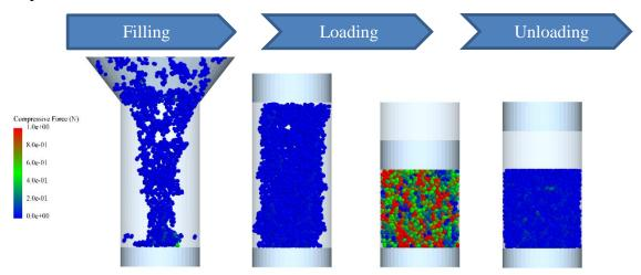
Figure 1. Snapshot of a DEM simulation for particles clipped up to the middle plane in an indie uniaxial compression test, EDEM (Altair Engineering)
