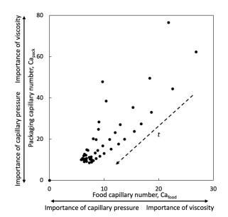
Figure 1. Experimental food capillary number against packaging capillary number, t = time
