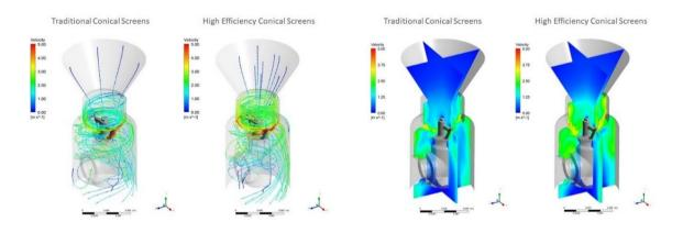
Figure 1. Air Flow (left) and Mass Flow (right) Across Traditional vs. New Hole
