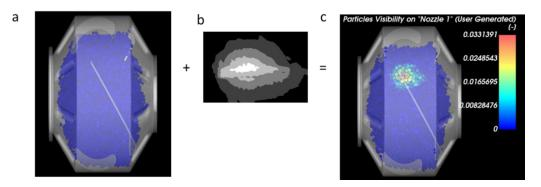
Figure 1. (a) Tablets in a drum coater, (b) spray distribution contour, and (c) snapshot of coated tablets with spray.
