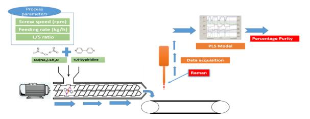
Figure 1. Equipment set-up, process parameters and process tools for measuring the purity of the MOF
