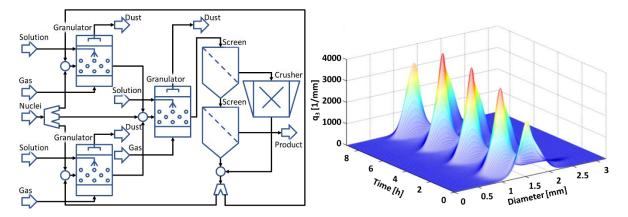
Figure 1. An example flowsheet of a two-stage granulation process with external classification and milling (left) and a time-dependent change in particle size distribution of granules (right).
