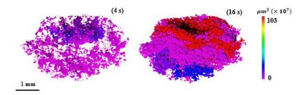
Figure 1. 3D pores volume rendering over time for 50% MCC-50% APAP.
