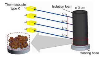
Figure 1. Experimental set up for heat transfer via conduction on moist particle bed
