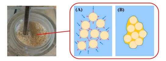
Figure 1. Lump formation during reconstitution, (A) particles start to swell (red arrows) due to water contact (blue arrows); (B) formation of a viscous outer layer leading to the aggregation of swelling particles
