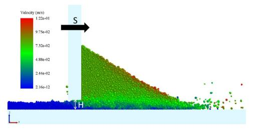
Figure 1. Illustration of powder spreading in EDEM
