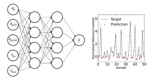
Figure 1. Artificial neural network for the prediction of solid moisture content based on process parameters bed temperature  $\vartheta_p$ , temperature of fluidization and exhaust gas  $\vartheta_{g,in}$  and  $\vartheta_{g,out}$  and moisture content of fluidization and exhaust gas  $Y_{in}$  and  $Y_{out}$ . The topology is shown on the left and a prediction on random samples of a batch dying of Cellets®200 is shown on the right.
