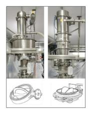
Figure 1. Refillers: TT-refiller (left), G-refiller (right).
