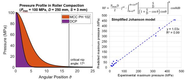
Figure 1. Pressure profile of microcrystalline cellulose and dicalcium phosphate in roller compaction (left), and the experimental  $P_{\text{max}}$  vs predicted  $P_{\text{max}}$  using the simplified Johanson model (right).
