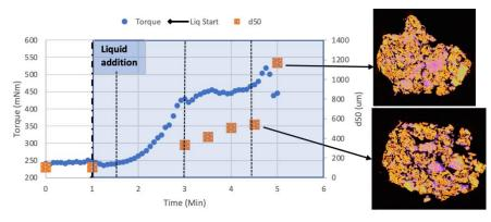
Figure 1. Dynamic median diameter overlayed with torque profile and microstructure images
