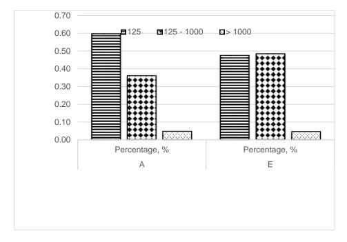
Figure 1. GSD comparison using crystalline PEG (A) versus amorphous PEG (E)
