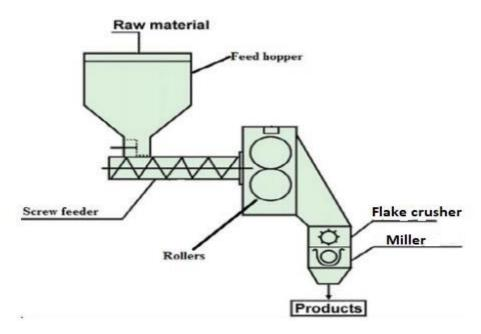
Figure 1. Diagram shows the main parts of roller compactor machine [2]
