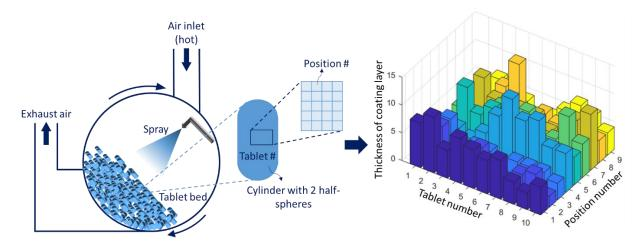
Figure 1. A schematic diagram for analyzing the tablet coating thickness.
