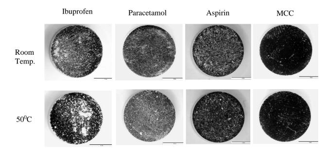
Figure 1. Microscopic images of powder sticking to punch surface at room and elevated temperature.
