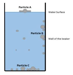
Figure 1. The problem faced when suspending solid particles into liquid. Particle A is floating on the liquid surface. Particle B is sticking on the wall of the beaker. While particle C settles down to the bottom.
