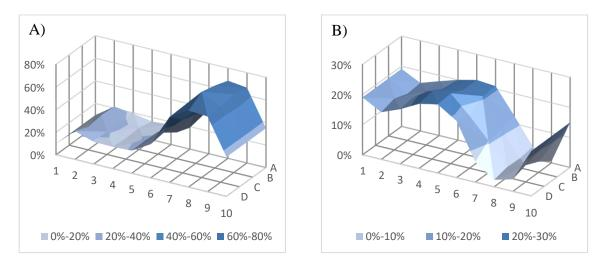
Figure 1. Dependency of different sieve fractions in a PSD on the position under the sieve mill in a roller compactor. A) sieve fraction <0.20 mm, B) sieve fraction 0.40 to 0.63 mm.
