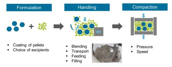
Figure 1. Illustration of influences on pellet coating integrity over a typical tabletting process chain
