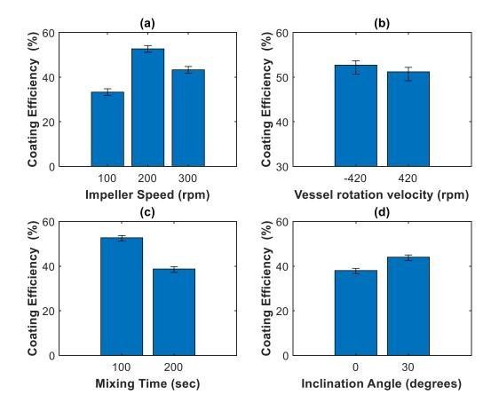
Figure 1. Influence of process variable on coating efficiency.
