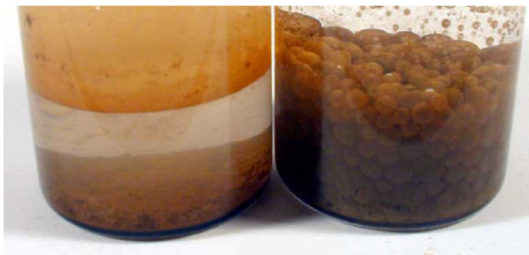
Fig. 7. Photograph showing the distribution of goethite in water/TCE/additive systems. The bottle on the left contains CTAB as an additive and the one on the right contains octadecylamine.
